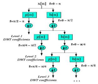
The signal is then subsampled by 2 since half of the number of samples are redundant. This doubles the scale. This procedure can mathematically be expressed as
